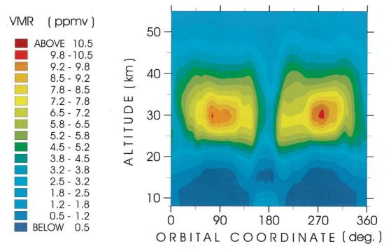
Fig. 2. Ozone distribution along the orbit selected for the retrieval test. VMR values are represented by different colors as a function of altitude and orbital coordinate. (ppmv, Parts in 10<sup>6</sup> by volume.)
