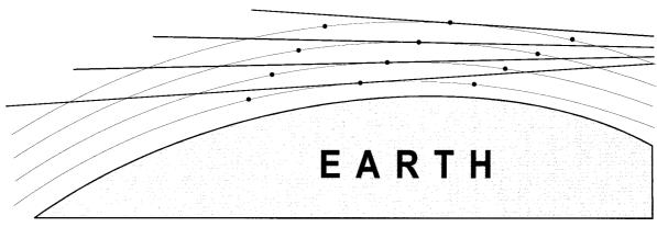
Fig. 1. Lines of sight for a satellite experiment that measures the atmosphere while looking backward along the track of the orbit. The tangent points of the limb-scanning sequence, plus those of two adjacent sequences, are marked by filled circles.
