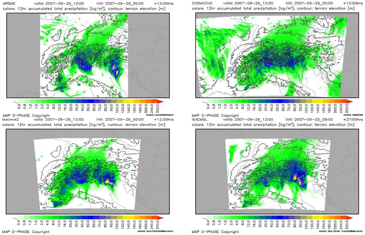
Figure 4: 12-h accumulated precipitation (mm) at 12 UTC, 26 Sep. 2007, as forecasted by AROME (top-left), COSMO\_CH (top-right), MOLOCH\_ECMWF (bottom-left) and MOLOCH\_GFS (bottom-right)
