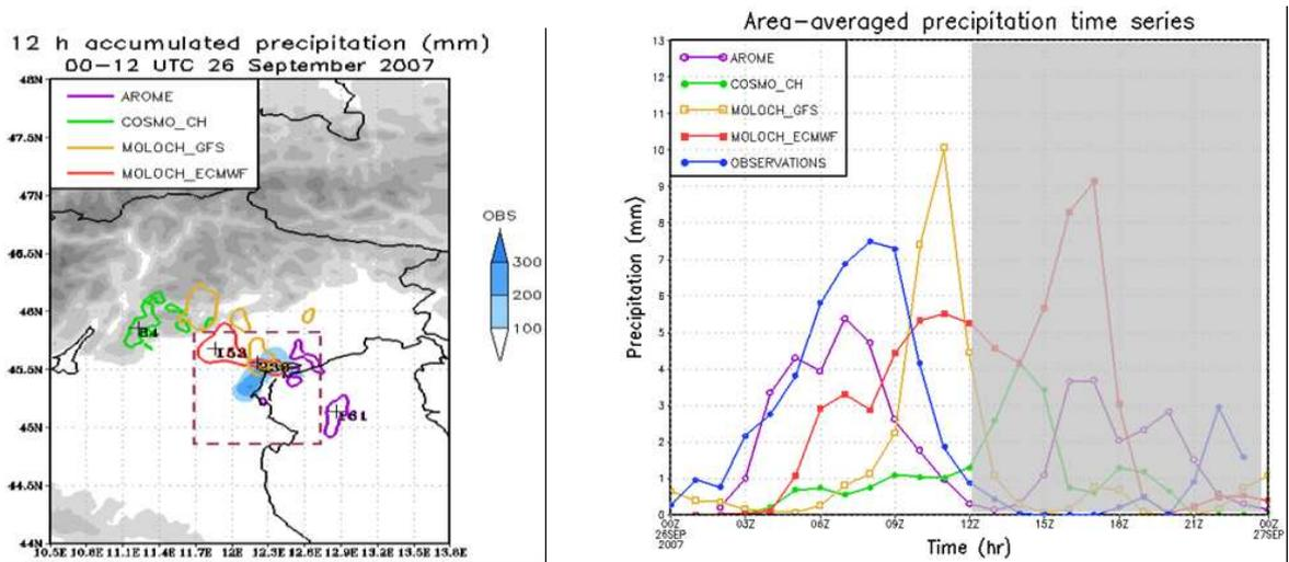
Figure 5: Left: 12-h observed (shaded) and simulated accumulated precipitation (mm), showing maximum amounts: 100 mm isoline for AROME and MOLOCH, 50 mm isoline for COSMO\_CH. Right: hourly precipitation time series averaged over the  $1^\circ \times 1^\circ$  domain depicted in the left panel
