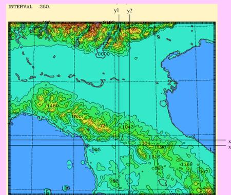
MOLOCH domain of integration, topography and land-sea mask. Contour interval 250 m. The position of the cross-sections is identified by thick lines.
