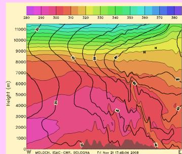
Saturated equivalent potential temperature (color) and pseudo angular momentum  $M = \mathbf{v} \times \mathbf{f}$  (thick contours) at 09:00 UTC section x2
