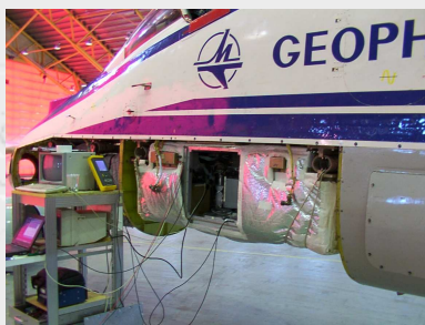
The SAFIRE/A spectrometer after installation onboard the M55 Geophysica stratospheric aircraft
