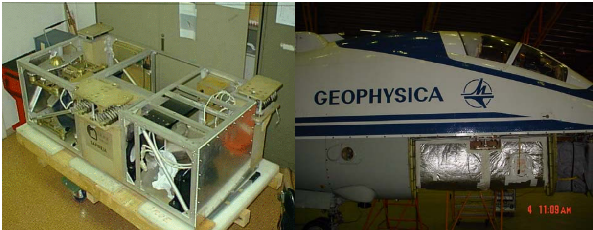
Figure 2.1: SAFIRE-A and the instrument onboard the M55 Geophysica.
