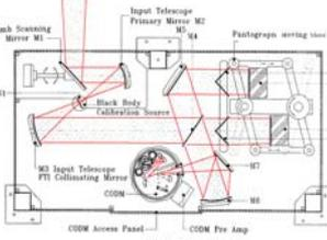
Figure 2: Schematic of the SAFIRE-A optical layout.
